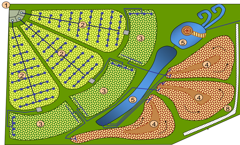
Fig. 2. Sketch of the 'butterfly' wastewater treatment system at Koh Phi Phi Don. (1) Distribution tanks with siphons; (2) vertical flow constructed wetland cells with distribution systems, (3) horizontal flow constructed wetland cells, (4) surface-flow constructed wetland cells, and (5) polishing ponds.
